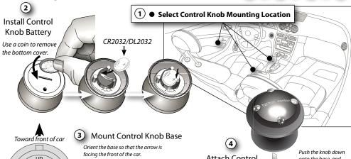
You can either screw the base to the mounting location or use the supplied adhesive pad.
