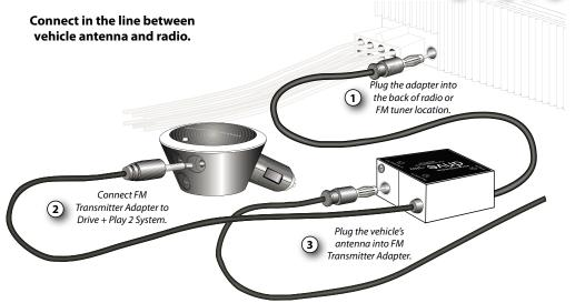
If your car's audio system does not provide an auxiliary input and there is no third-party adapter available, use the Drive + Play 2 system's wired FM Antenna Adapter for the best audio performance.
